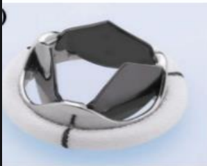
provides flow characteristics that more closely mimic native aortic valve-like leaflets to close before flow reverses, a phenomenon that is not seen in the current generation of prosthetic valves. (a) Valve from above in fully open position. (b) Elevated isometric view of the valve in a fully open position. (c) Valve with three pyrolytic carbon leaflets and ring. Images are courtesy of Ulrich Steinseifer, Helmholtz Institute, Aachen University.
